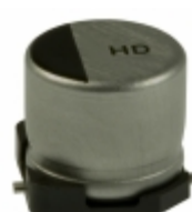
EEV-HD1H100P Panasonic Electronic Components CAP ALUM 10UF 20% 50V SMD
