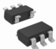
MCP73832T-4ADI/OT Microchip Technology IC CONTRLR LI-ION 4.40V SOT23-5
