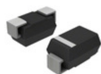
SMBJ30E3/TR13 Microsemi Corporation TVS DIODE 30VWM 53.5VC SMBJ
