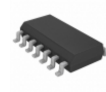
PIC16LF1704T-I/SL Microchip Technology IC MCU 8BIT 7KB FLASH 14SOIC
