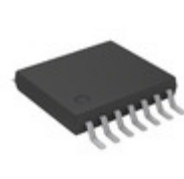
PIC16LF1704T-I/ST Microchip Technology IC MCU 8BIT 7KB FLASH 14TSSOP
