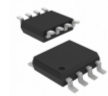
CY14MB064J1-SXI Cypress Semiconductor Corp IC NVSRAM 64KBIT 3.4MHZ 8SOIC
