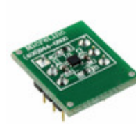
MIC94355-4YMT-EV Micrel / Microchip Technology EVAL BRD 1.2V 500MA LDO MIC94355
