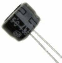
ECE-A1CK101Q Panasonic Electronic Components CAP ALUM 100UF 20% 16V RADIAL
