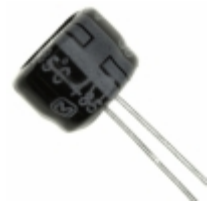
ECE-A1CK101I Panasonic Electronic Components CAP ALUM 100UF 20% 16V RADIAL
