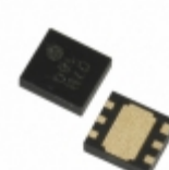
XC6123F628ER-G Torex Semiconductor Ltd IC WATCHDOG TIMER 6-USP
