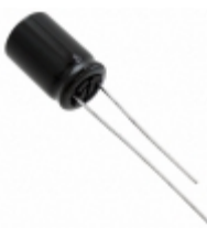
EEU-TP1E331B Panasonic Electronic Components CAP ALUM 330UF 20% 25V RADIAL
