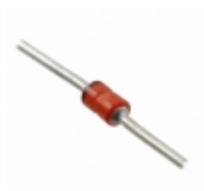
MP5KE60CAE3 Microsemi Corporation TVS DIODE 60VWM 96.8VC DO41
