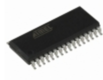
AT28C010-20SI Microchip Technology IC EEPROM 1MBIT 200NS 32SOIC
