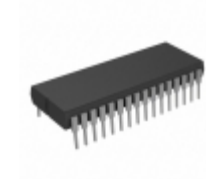
AT28C010-25DM/883 Micrel / Microchip Technology IC EEPROM 1M PARALLEL 32CDIP
