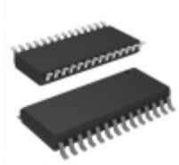
HI5767/4CBZ Intersil CONV A/D 10BIT 40MSPS 28-SOIC
