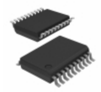
PIC24FV08KM101T-I/SS Microchip Technology IC MCU 16BIT 8KB FLASH 20SSOP
