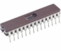
PIC16C63A/JW Microchip Technology IC MCU 8BIT 7KB EPROM 28CDIP
