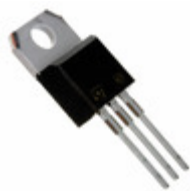
BUL49D STMicroelectronics TRANS NPN 450V 5A TO-220
