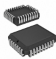
AT29C257-70JI Microchip Technology IC FLASH 256KBIT 70NS 32PLCC
