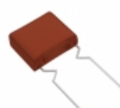
ECW-F2184HAQ Panasonic Electronic Components CAP FILM 0.18UF 3% 250VDC RADIAL
