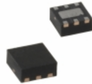
MIC5319-1.85BML-TR Microchip Technology IC REG LDO 1.85V 0.5A 6MLF
