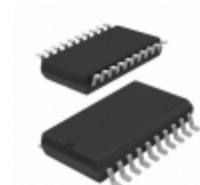
AT89S4051-24SU Microchip Technology IC MCU 8BIT 4KB FLASH 20SOIC
