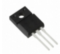
BA033T Rohm Semiconductor IC REG LDO 3.3V 1A TO220FP
