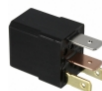
CM1AF-12V Panasonic Electric Works RELAY AUTOMOTIVE SPST 35A 12V
