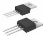
IXFP26N30X3 IXYS Corporation 300V/26A ULTRA JUNCTION X3-CLASS
