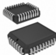
AT28HC64B-70JI Microchip Technology IC EEPROM 64KBIT 70NS 32PLCC
