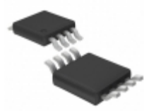
LTC1475CMS8#TRPBF Linear Technology IC REG MULT CONFIG INV ADJ 8MSOP
