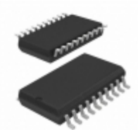
MC33883DW NXP Semiconductors / Freescale IC H-BRIDGE PRE-DRIVER 20- SOIC
