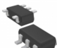
XC6123D731MR-G Torex Semiconductor Ltd IC WATCHDOG TIMER SOT-25
