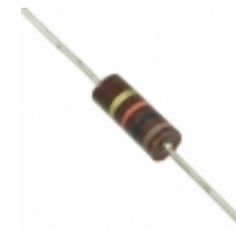
RC12JB100K Stackpole Electronics Inc. RES 100K OHM 1/2W 5% AXIAL
