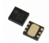
XC6121C244ER-G Torex Semiconductor Ltd IC WATCHDOG TIMER 6-USP
