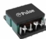
PH0814CNLT Pulse Electronics Corporation XFMR, ER19 PLANAR, 5:6:2:1, SMT
