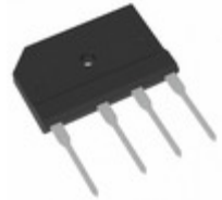
TS35P06GHC2G TSC (Taiwan Semiconductor) BRIDGE RECT 1P 800V 35A TS-6P
