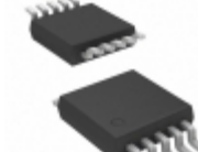
MCP4652-104E/UN Microchip Technology IC DGTL POT 100K 257TAPS 10-MSOP
