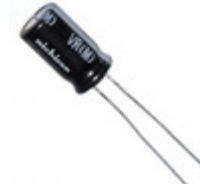
UVR1H330MDD1TD Nichicon CAP ALUM 33UF 20% 50V RADIAL
