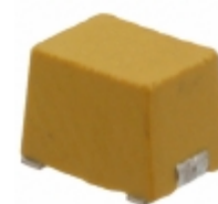
IMC1812ER4R7K Vishay Dale FIXED IND 4.7UH 315MA 1 OHM SMD
