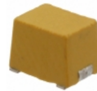
IMC1812ER470K Vishay Dale FIXED IND 47UH 140MA 5 OHM SMD
