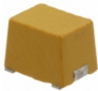
IMC1812ER3R3K Vishay Dale FIXED IND 3.3UH 355MA 800 MOHM
