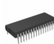
AT28C010-15DM/883 Micrel / Microchip Technology IC EEPROM 1M PARALLEL 32CDIP
