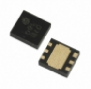
XC6122D519ER-G Torex Semiconductor Ltd IC WATCHDOG TIMER 6-USP
