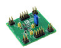
ADP7156CP-3.3EVALZ ADI (Analog Devices, Inc.) EVAL BOARD FOR ADP7156
