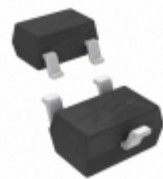
ZUMT618TA Diodes Incorporated TRANS NPN 20V 1.25A SC70-3
