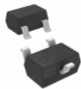
ZUMT591TA Diodes Incorporated TRANS PNP 60V 1A SC70-3
