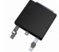
DGS19-025CS IXYS DIODE SCHOTTKY 250V 31A TO252AA
