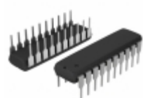
PIC24F16KA301-E/P Micrel / Microchip Technology IC MCU 16BIT 16KB FLASH 20DIP
