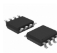
MCP6L72T-E/SN Microchip Technology IC OPAMP GP 2MHZ RRO 8SOIC
