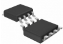
LTC1261CS8-4.5#PBF ADI (Analog Devices, Inc.) IC REG SWTCHD CAP INV 12MA 8SOIC
