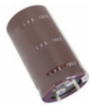
ELXS451VSN471MA45S United Chemi-Con CAP ALUM 470UF 20% 450V SNAP
