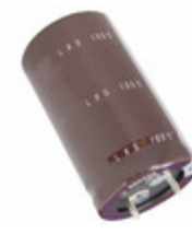
ELXS451VSN391MA35W United Chemi-Con CAP ALUM 390UF 20% 450V SNAP
