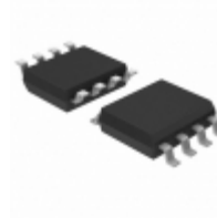
AT25256W-10SC-1.8 Microchip Technology IC EEPROM 256KBIT 2.1MHZ 8SOIC
