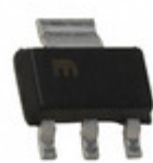
MIC5239-5.0BS Microchip Technology IC REG LDO 5V 0.5A SOT223
