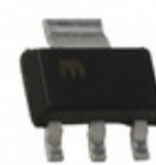
MIC5239-3.3YS-TR Microchip Technology IC REG LDO 3.3V 0.5A SOT223
