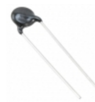
ERZ-E07A561 Panasonic Electronic Components VARISTOR 560V 2.5KA DISC 9MM
