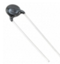
ERZ-E07A511CS Panasonic Electronic Components VARISTOR 510V 2.5KA DISC 9MM
