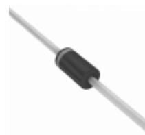
BZX85B6V2-TAP Vishay Semiconductor Diodes Division DIODE ZENER 6.2V 1.3W DO41
