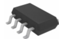
LTC2950CTS8-2#TRMPBF Linear Technology IC PB ON/OFF CONTROLLER TSOT23-8
