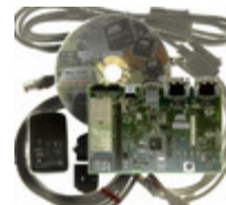
AT91SAM7XC-EK Micrel / Microchip Technology KIT EVAL FOR AT91SAM7XC256/128
