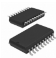
ADUM4151BRIZ Analog Devices Inc. DGTL ISOLATOR 5KV 7CH SPI 20SOIC
