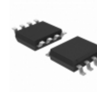
MCP6N11-001E/SN Microchip Technology IC OPAMP INSTR 500KHZ RRO 8SOIC
